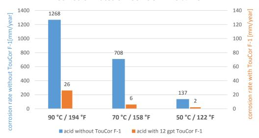
Test conditions: 13Cr80 specimen were treated at different temperatures for 6 h under stirring in 15 wt-% hydrochloric acid containing 12 gpt TouCor F-1. Reference tests were done using non-inhibited HCI.
